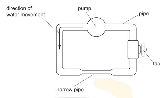
The diagram is a model of an electrical circuit.
